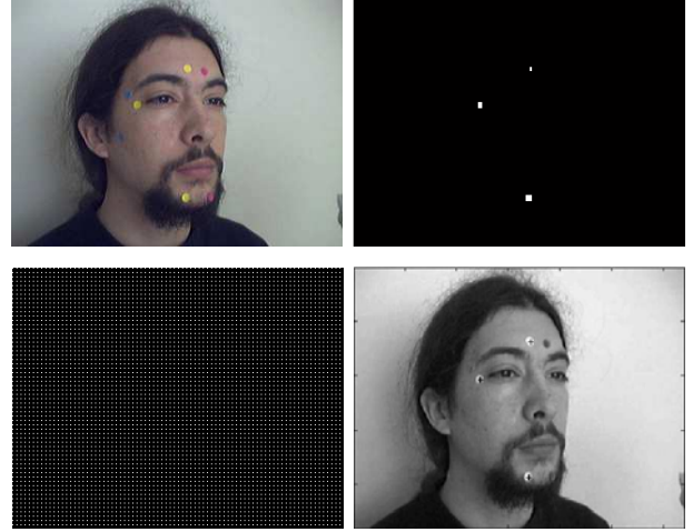
Figure 4. Yellow marker detection (reading left to right): original image, binary image after color filtering applied on Hue and Saturation components, a grid of white pixels, and marker coordinate localization.
